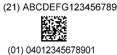
Figure 2.1.10-4. Example of GS1 DataMatrix symbol encoded with GTIN and serial number AI (21)
