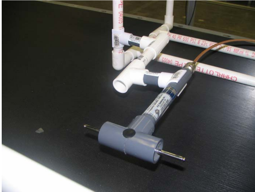
Figure 6 Fixture for Holding Probe Antenna
