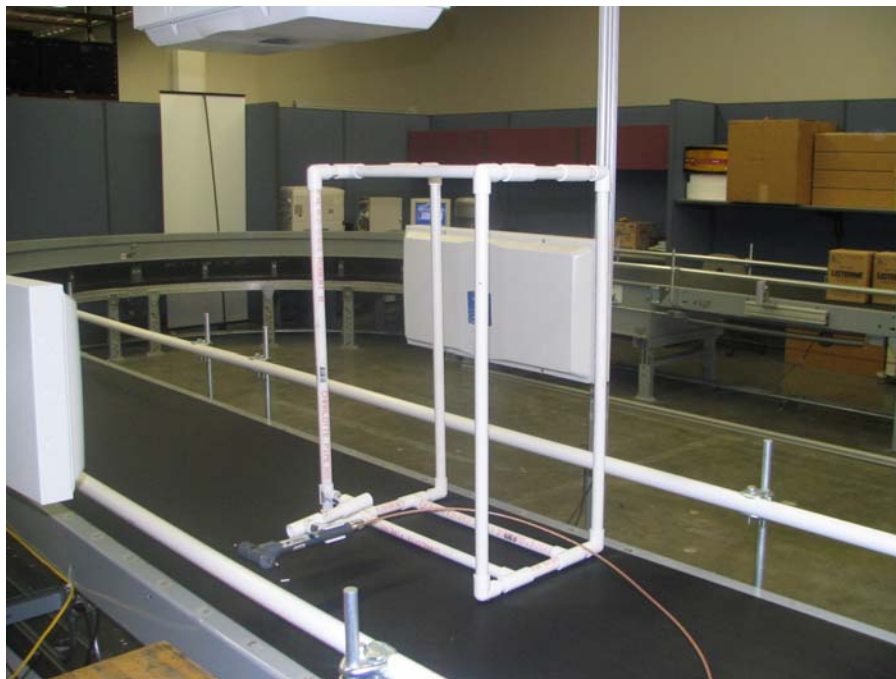
Figure 5 Probe antenna positioning
