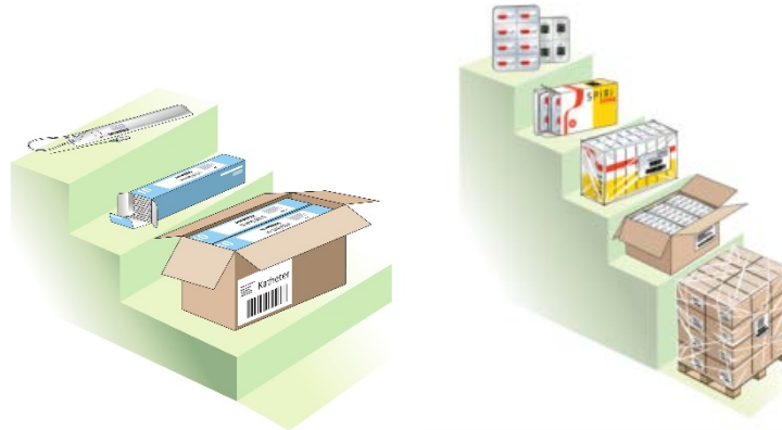
Figure B-1 Example of two products and their respective packaging hierarchy levels
