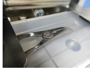
Fig. 4-12 Marking example No loss of product function
