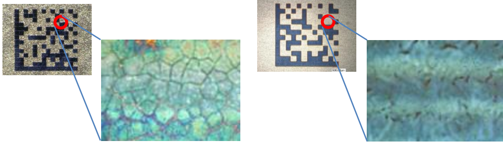
Fig. 4-3 Microscope magnification image (SUS) Left: Black marking Right: Cold marking
