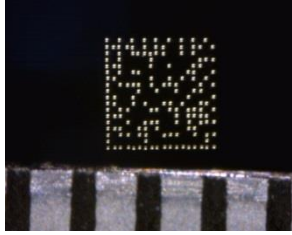
Fig. 4-8 Marking of 1.0 mm × 1.0 mm (Scale: 0.5 mm)
