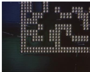
Fig. 4-9 Marking 1 cell with 2 × 2 dots
