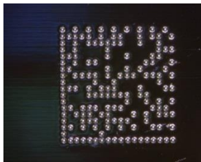
Fig. 4-10 Two-dimensional barcodes with different output sizes for 1 cell with 1 dot Automatically adjusts the size of the dot and the distance between dots. (Photos are taken at the same magnification.)
