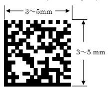
② In case of steel instruments in bar shape on which 3mm square space cannot be secured for marking
