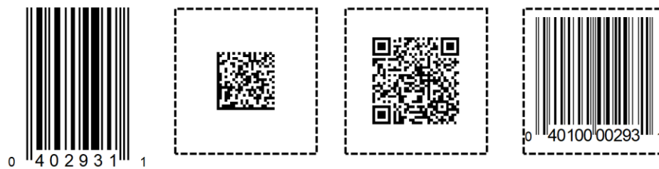
Figure 4-14. From left to right, UPC-E symbol sized at 0.264 millimetre (0.0104 inch), followed by a GS1 DataMatrix sized at 0.457 millimetre (0.0180 inch), a QR Code (GS1 Digital Link URI) sized at 0.457 millimetre (0.0180 inch) and a UPC-A 0.150 millimetre (0.0059 inch). The dotted lines indicate the space a UPC-E requires, including Quiet Zones.
