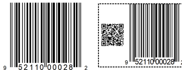
Figure 4-2 5 . UPC-A barcode with an X-dimension of 0.25 mm (0.010 inches) (left) versus a combination of a QR Code with GS1 Digital Link URI data sized at 0.25 mm (0.010 inches) and UPC-A symbol sized at 0.18 mm (0.007 inches) for placement within the same space (right). The dotted
