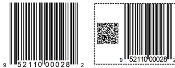
Figure 1-2 3 . UPC-A symbol sized at 0.264 millimetre (0.0104 inch) compared to a combination of a QR Code (GS1 Digital Link URI) sized at 0.264 millimetre (0.0104 inch) and UPC-A symbol sized at 0.169 millimetre (0.0067 inch) for placement within the same space. The dotted line indicates the space a UPC-A requires, including Quiet Zones.
