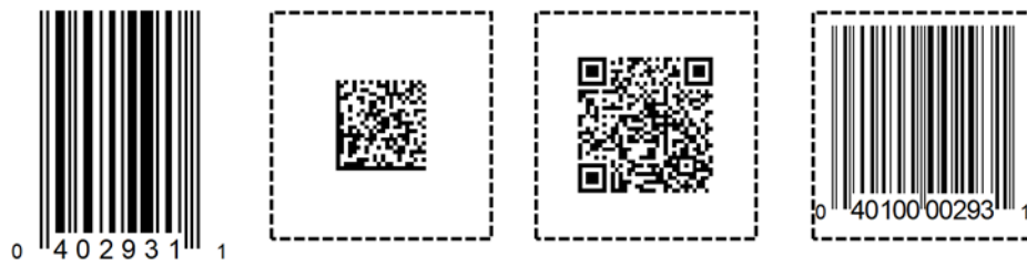
Figure 1-1 2 . From left to right, UPC-E symbol sized at 0.264 millimetre (0.0104 inch), followed by a QR Code (GS1 Digital Link URI) sized at 0.297 millimetre (0.0117 inch), a QR Code (GS1 Digital Link URI) sized at 0.396 millimetre (0.0150 inch) and a UPC-A sized at 0.140 millimetre (0.0055 inch). The dotted lines indicate the space a UPC-E requires, including Quiet Zones.
