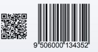
Independent of direction of travel the scanner transmits: 010950600013435210ABC^17231231 In this example, the "^" replaces the
