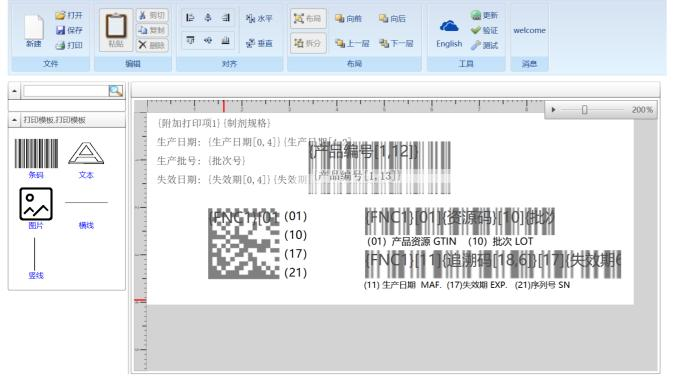
Figure 2: GS1 encoding and label template
